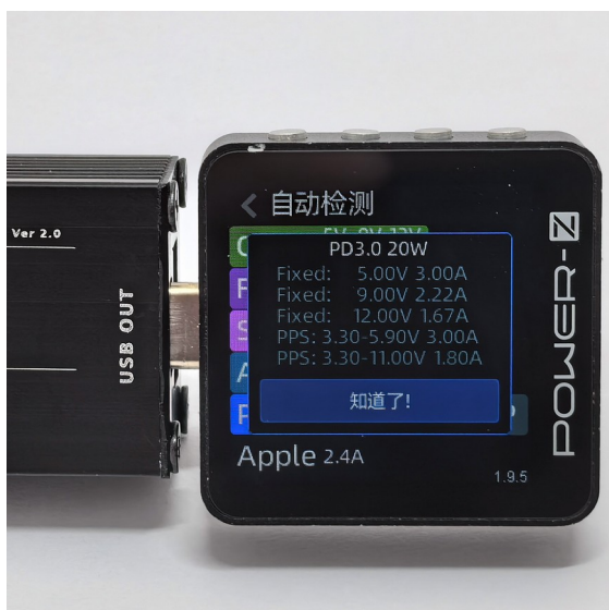
Power-Z test photos. Left: USB-C PD 3.0 profiles and both PPS ranges. Right: detected QC 2.0/3.0 voltage modes.
