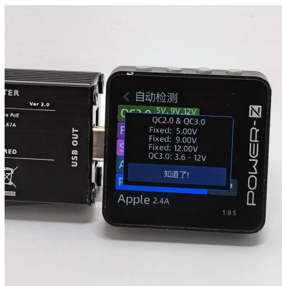
Power-Z test photos. Left: USB-C PD 3.0 profiles and both PPS ranges. Right: detected QC 2.0/3.0 voltage modes.
